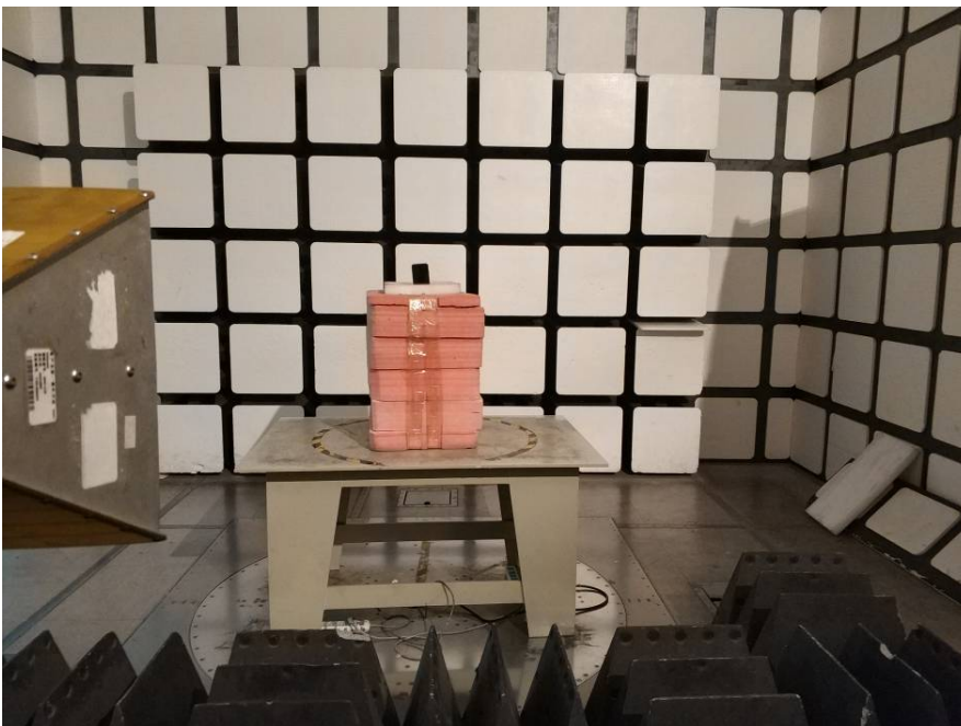
Radiated Emissions View (Above 1 GHz)
