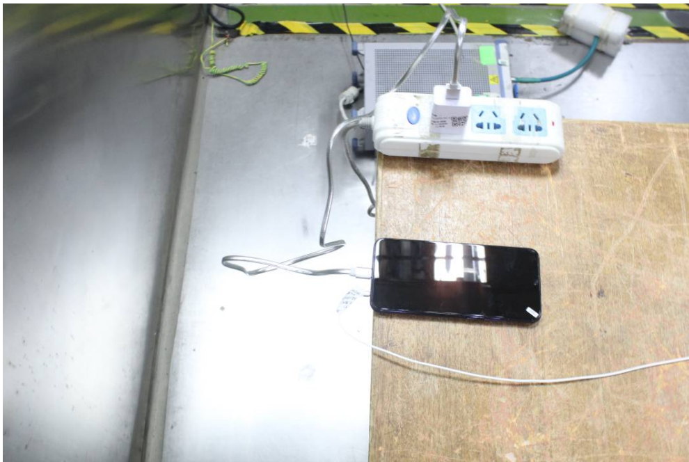
Conducted Emissions - Side View
