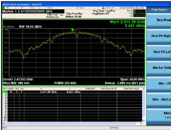
802.11b LOW CHANNEL, CARRIER LEVEL
