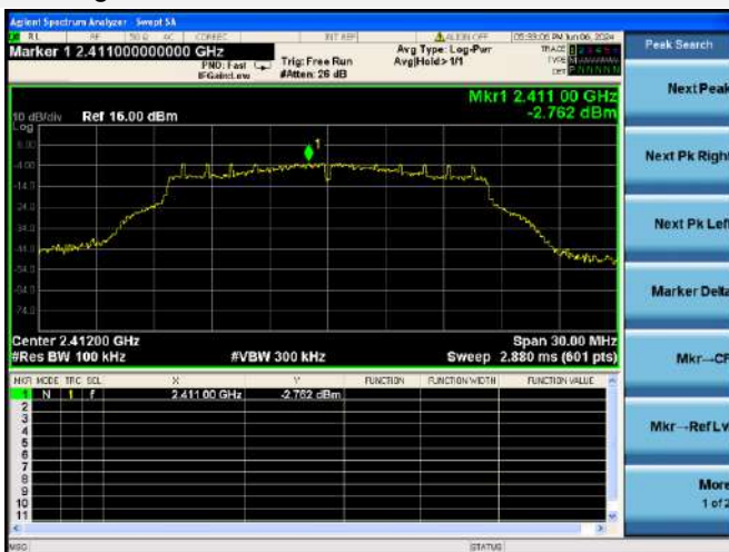
802.11g LOW CHANNEL, CARRIER LEVEL
