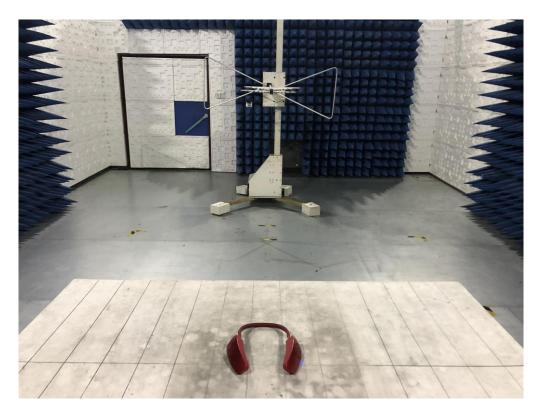
RADIATED EMISSION TEST SETUP ABOVE 1GHZ
