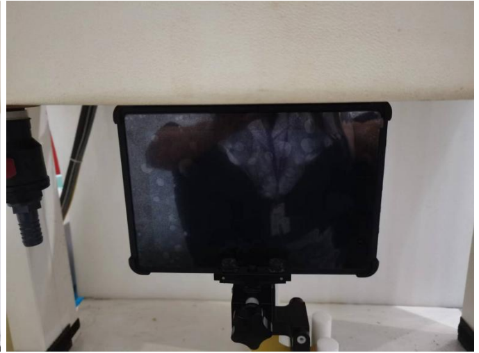
Fig-4.6 Bottom of EUT with 0 cm Gap (Body Mode)
