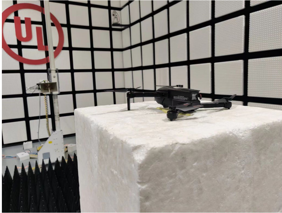
Radiated Disturbance Setup (Above 1 GHz – X axis)
