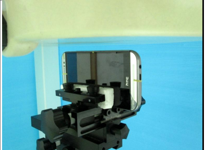
Right Side of EUT with 1.0 cm Gap
