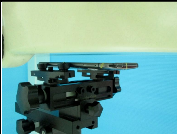
Front Face of EUT with 1.0 cm Gap
