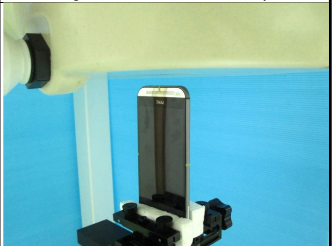
Bottom Side of EUT with 1.0 cm Gap
