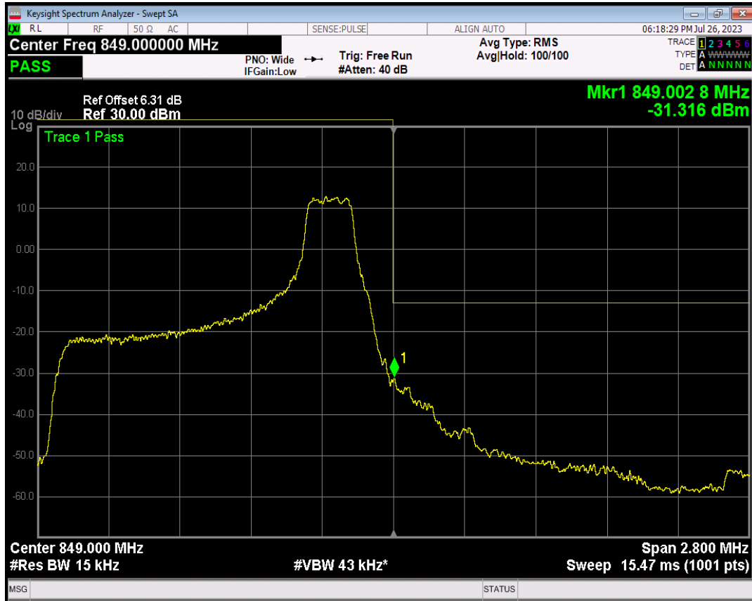
Band5 QPSK BW=1.4MHz Channel=20643 RB Size=6 Position=#0
