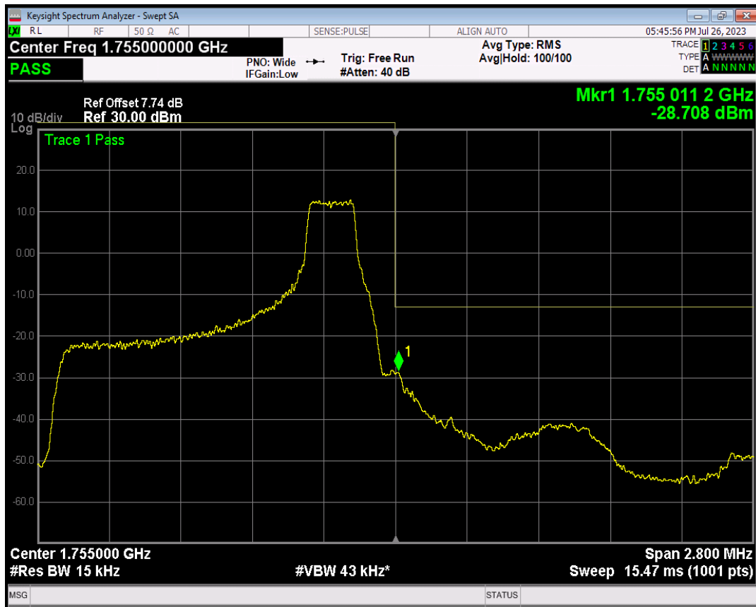
Band4 QPSK BW=1.4MHz Channel=20393 RB Size=6 Position=#0
