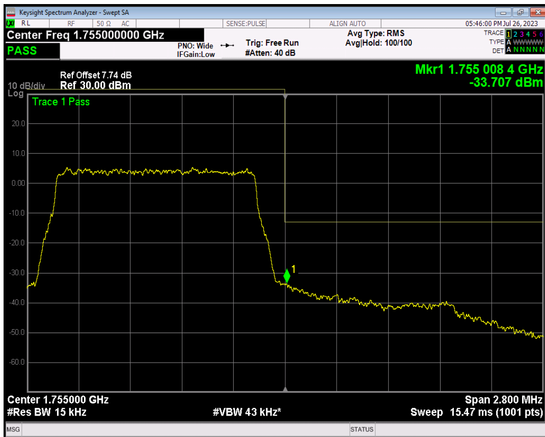
Band4 16QAM BW=1.4MHz Channel=20393 RB Size=1 Position=#0
