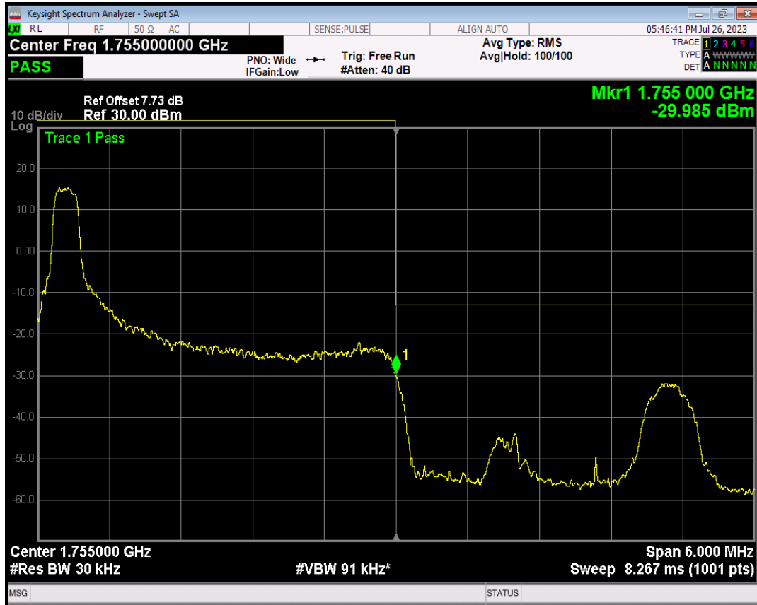
Band4 16QAM BW=3MHz Channel=20385 RB Size=1 Position=#Max
