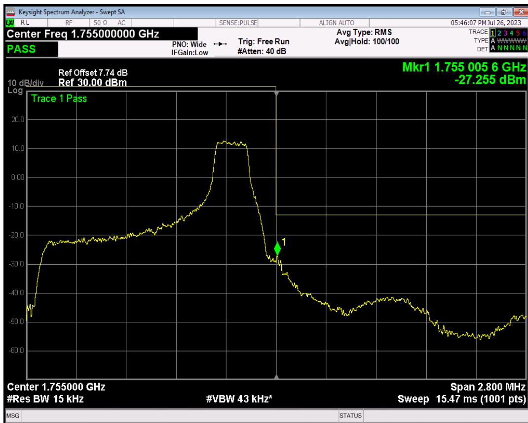
Band4 16QAM BW=1.4MHz Channel=20393 RB Size=6 Position=#0
