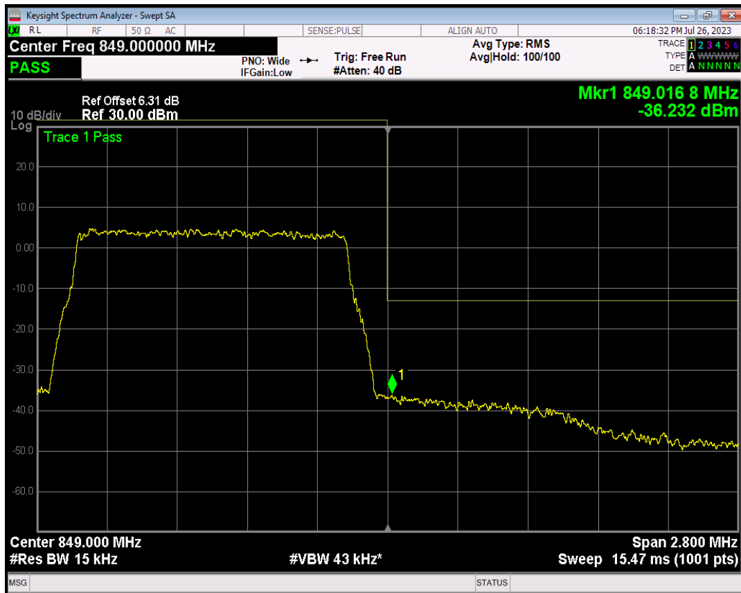
Band5 16QAM BW=1.4MHz Channel=20643 RB Size=1 Position=#0
