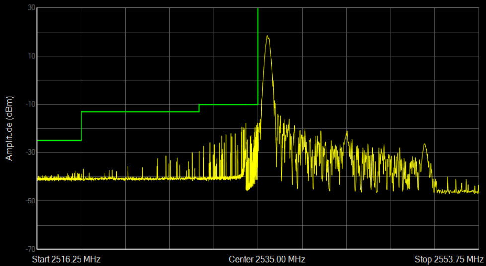
Band41(2535-2655) QPSK BW=15MHz Channel=40115 RB Size=1 Position=#0
