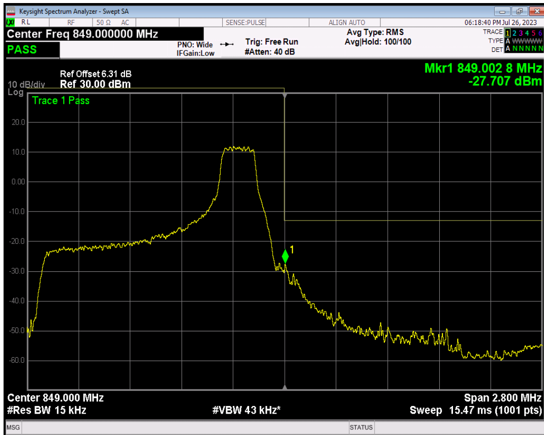
Band5 16QAM BW=1.4MHz Channel=20643 RB Size=6 Position=#0
