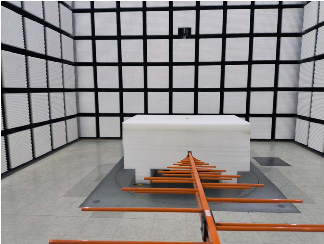
Radiated Emission Above 1GHz View
