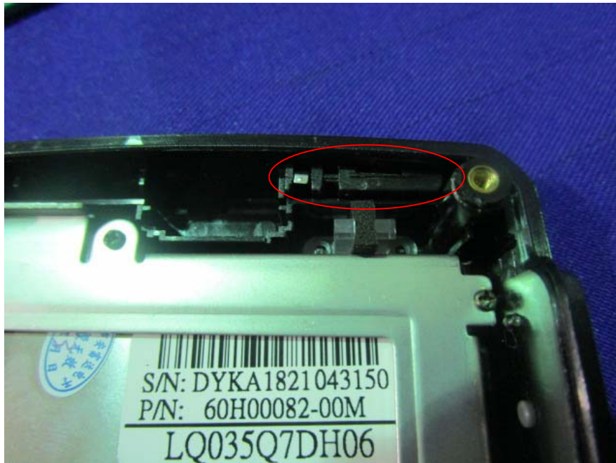
EUT – BT/Wifi Antenna Location View
