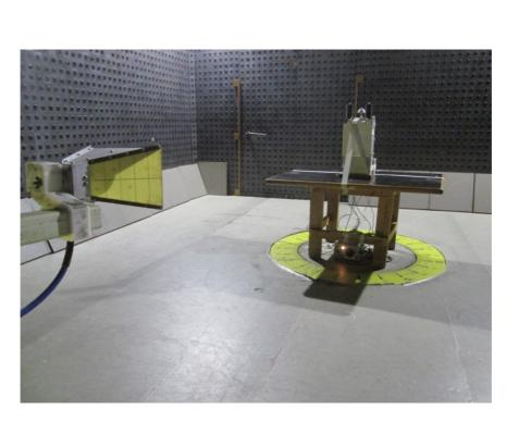
Photograph No.5 Spurious emissions measurement setup in the anechoic chamber in 1 – 18 GHz
