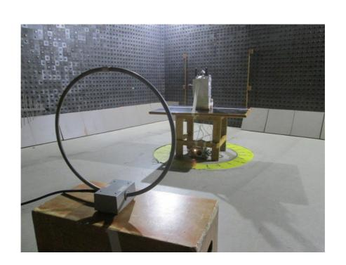
Photograph No.3 Spurious emissions measurement setup in the anechoic chamber below 30 MHz
