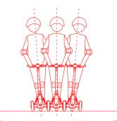
5. Power on the turn signal before turn. To turn, shift your body weight and turn the handle slightly. Power off when turn finished.
