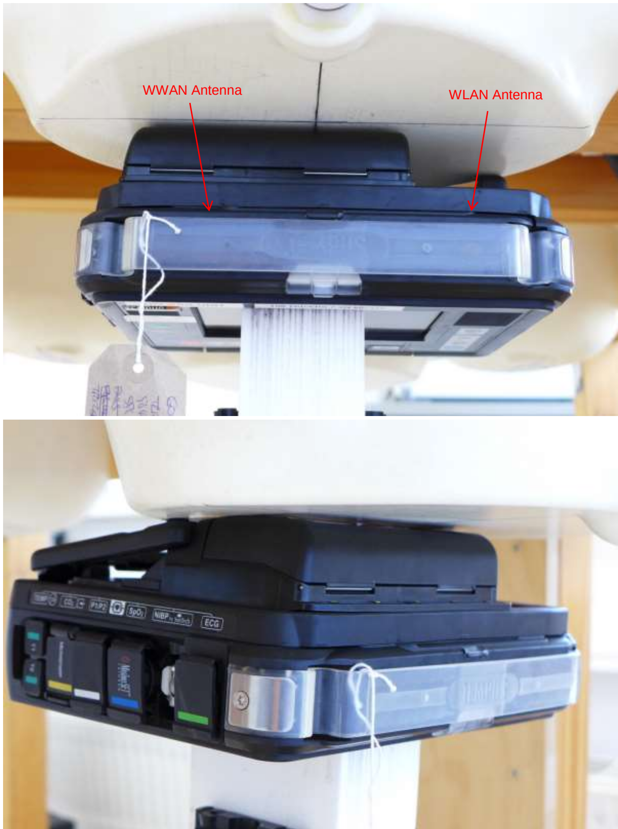
Pic. 3: Test position, back side of DUT towards the phantom, 0 mm distance.
