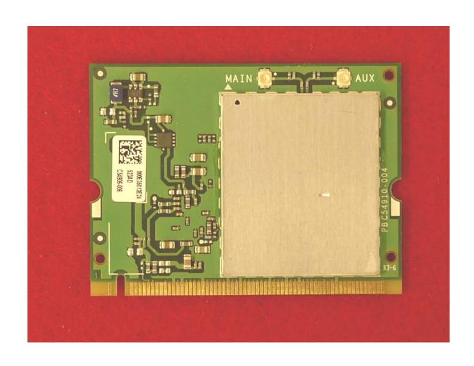
Top View of the WLAN Transmitter "Insulation Removed"
