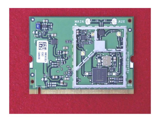
Top View of the WLAN Transmitter "Shielding Removed"
