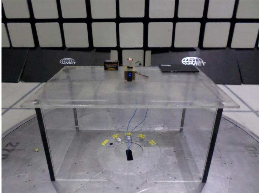
**Photograph 1. Radiated Emissions, Setup Below 1GHz, Front view**
