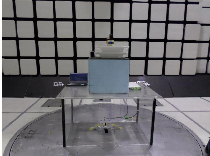
**Photograph 3. Radiated Emissions, Setup Above 1GHz, Front view**
