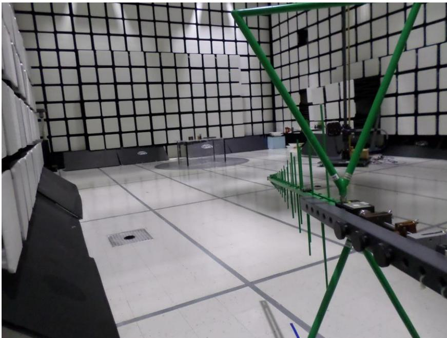
**Photograph 2. Radiated Emissions, Setup Below 1GHz, Antenna view**
