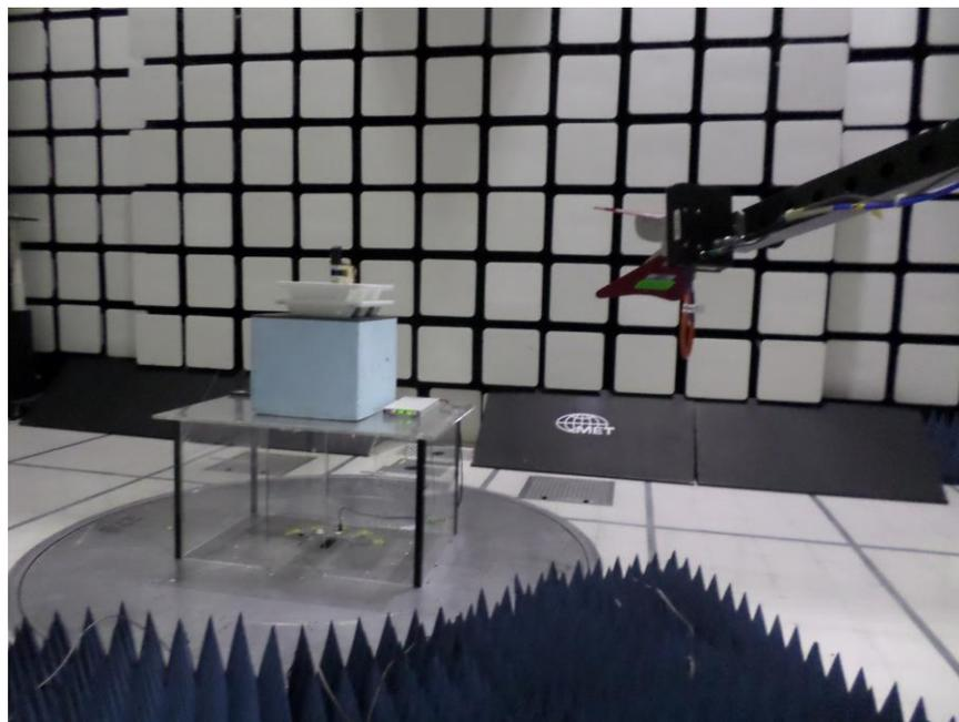
**Photograph 4. Radiated Emissions, Setup Above 1GHz, Antenna view**
