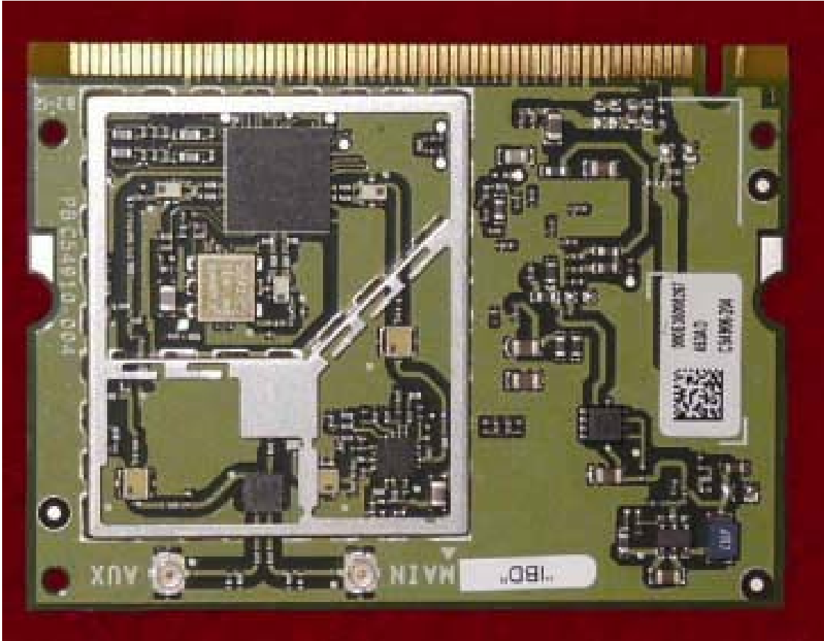
Front with Shielding Removed
