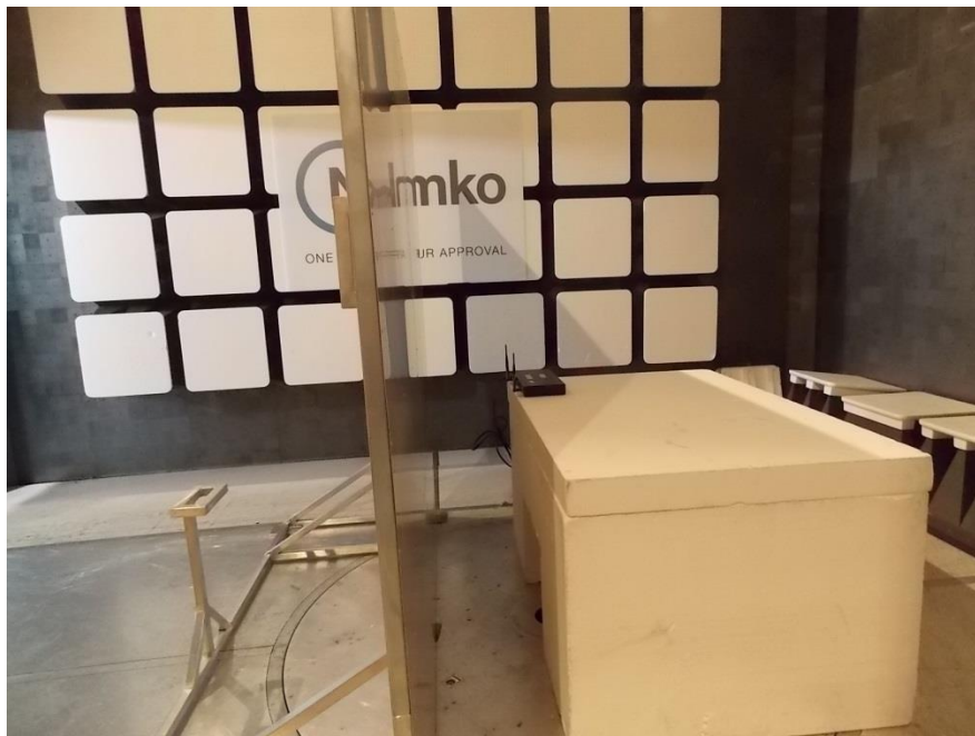
Figure 8.1-4: AC power line conducted emissions limits setup photo
