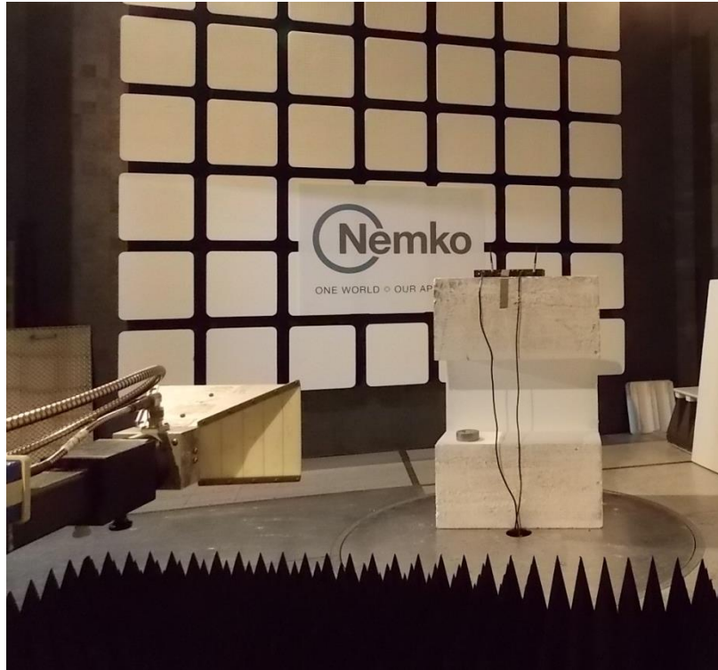
Figure 8.4-15: Radiated spurious (out-of-band) emissions setup photo – above 1 GHz
