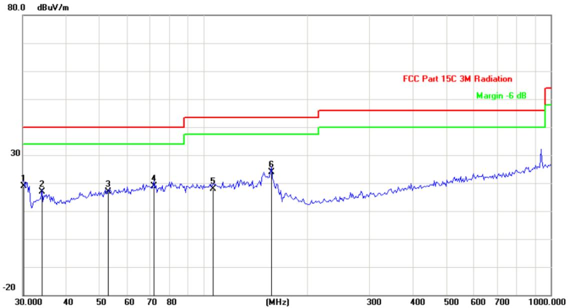
Site: Polarization: *Horizontal* Temperature: 25
