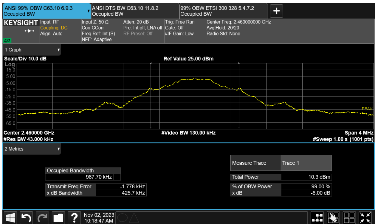
Figure TR03.2: Bandwidth data for ANT at channel (2460 MHz)
