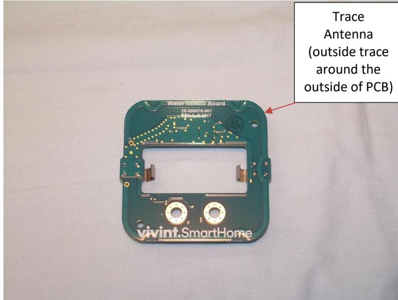
**Photograph 5 – View of the Bottom Side of the EUT PCB**
