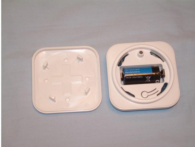
**Photograph 1 – Top Removed from the EUT**
