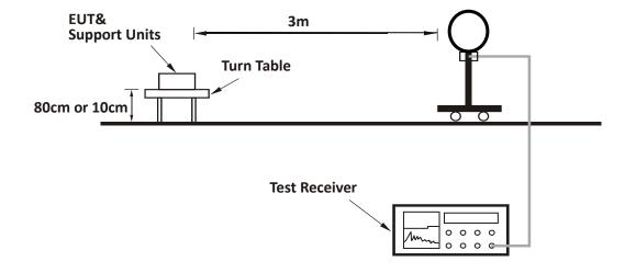
For Radiated emission 30MHz to 1GHz:
