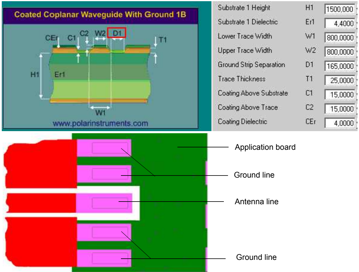
Figure 15: Micro-Stripline on 1.5mm Standard FR4 PCB - example 1
