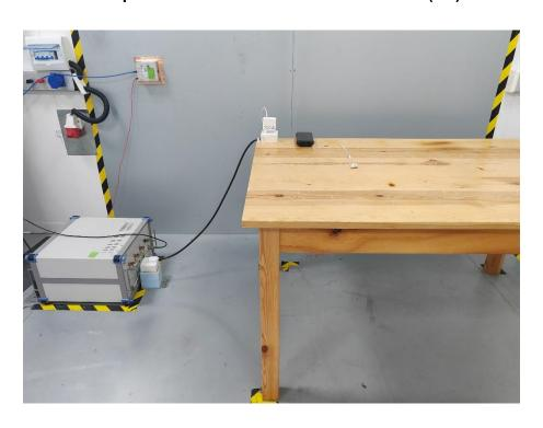
Set-up for Radiated Emission (RE), Below 1GHz
