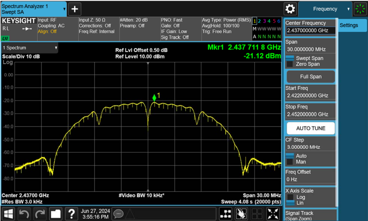
Figure 14: Power Spectral Density, 802.11b, 2437MHz
