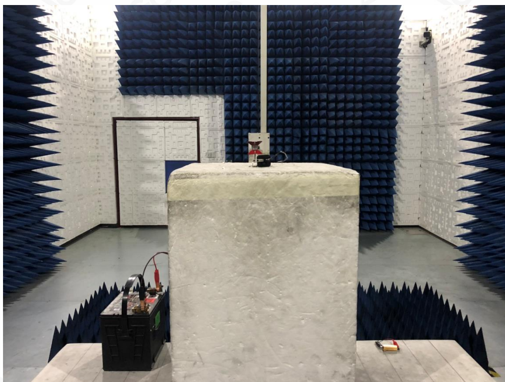
RADIATED EMISSION TEST SETUP ABOVE 1G
