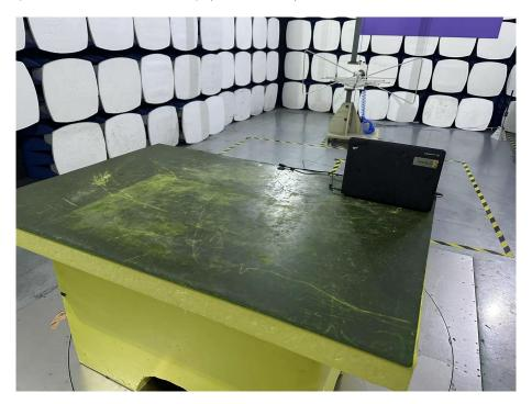
Spurious Emission Test Setup (Above 1GHz)
