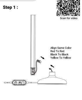
Connect the wire interface between the lamp base and led tube 4
