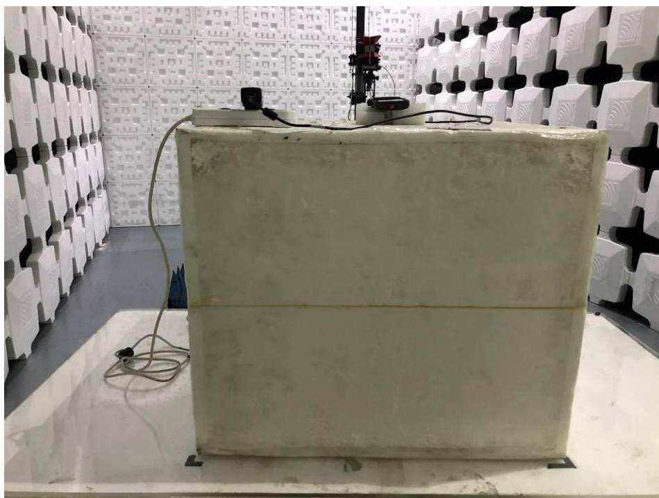
Fig. 4 Power line conducted emission setup photo
