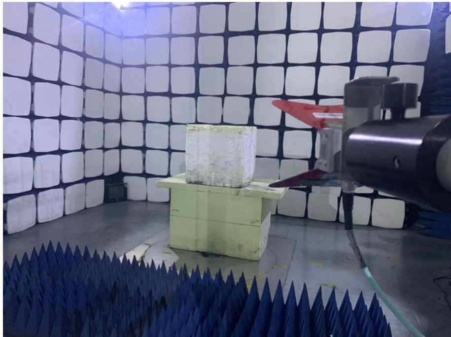
Radiation Emission Test Setup (1GHz to 18GHz)
