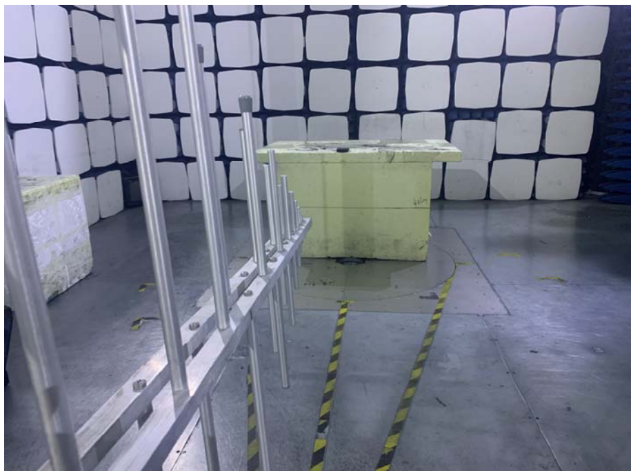
Radiation Emission Test Setup (30MHz to 1GHz)
