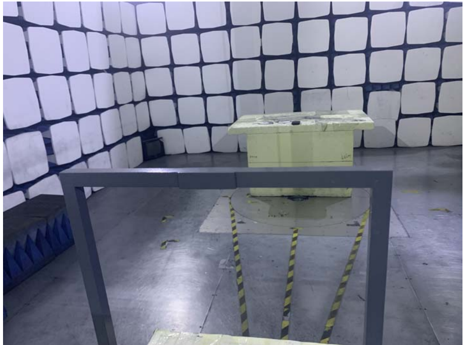
Radiation Emission Test Setup (Below 30MHz)
