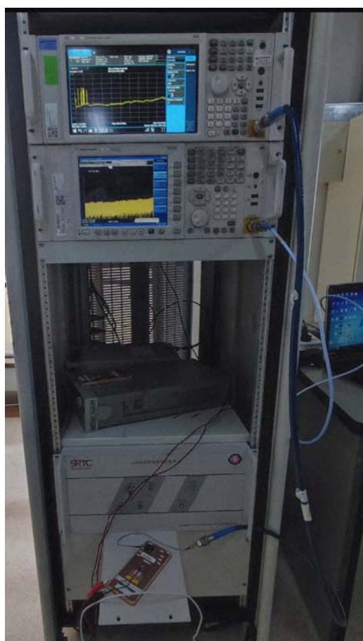
RF Conducted Test setup (BT/WIFI)
