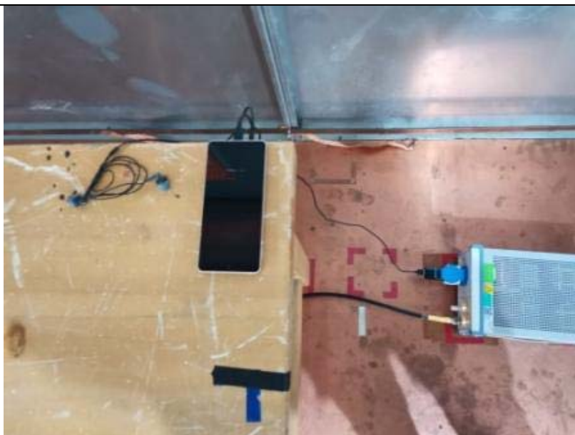
Conducted Emissions Test Setup (with charger)
