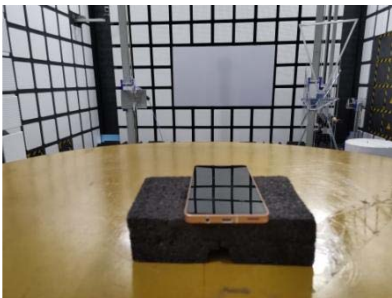
Spurious Radiated Emissions Test setup
