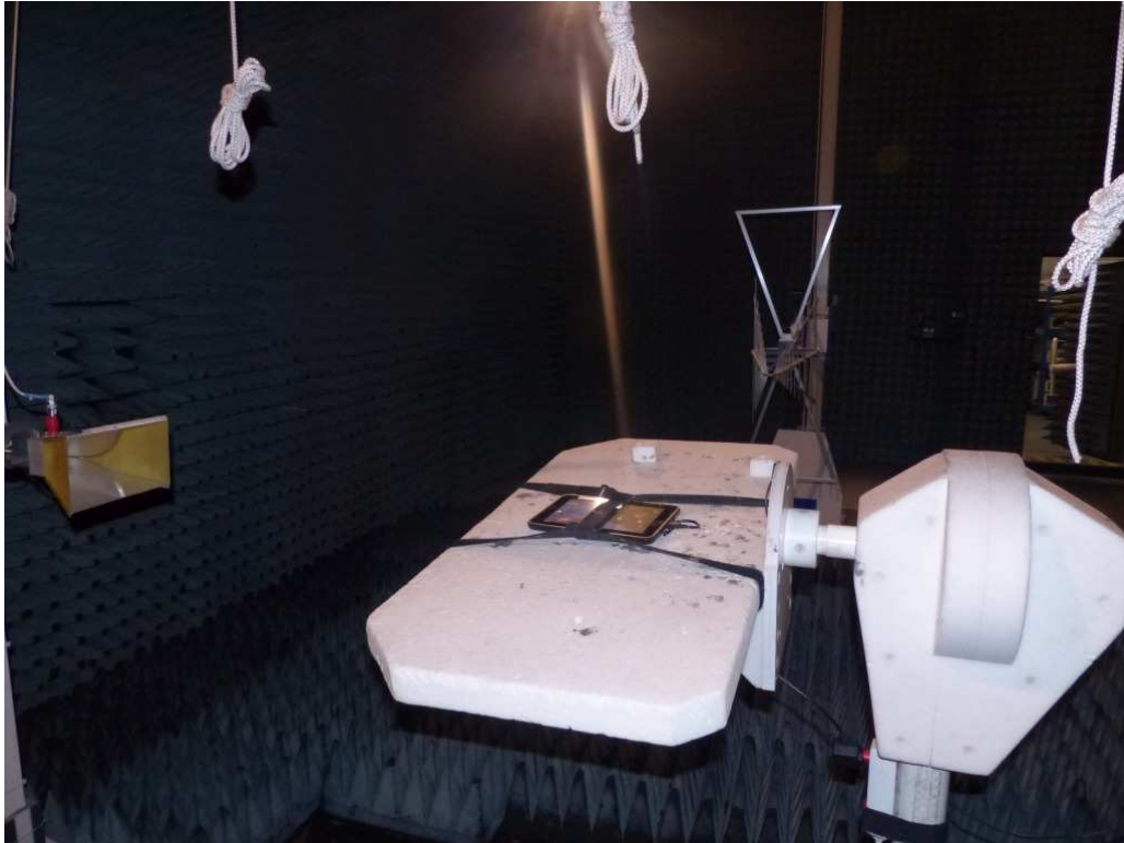
Photo 3: Test setup for radiated measurements (Enclosure, fully-anechoic chamber, 1-18 GHz intentional radiator §15.247 / 1-15 GHz intentional radiator §15.407)
