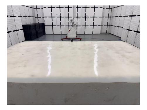
Set-up for Radiated Spurious Emission, Above 1GHz
