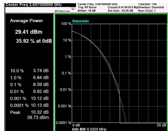
Channel: TOP, Modulation: 256QAM, BW=5MHz, CCDF
