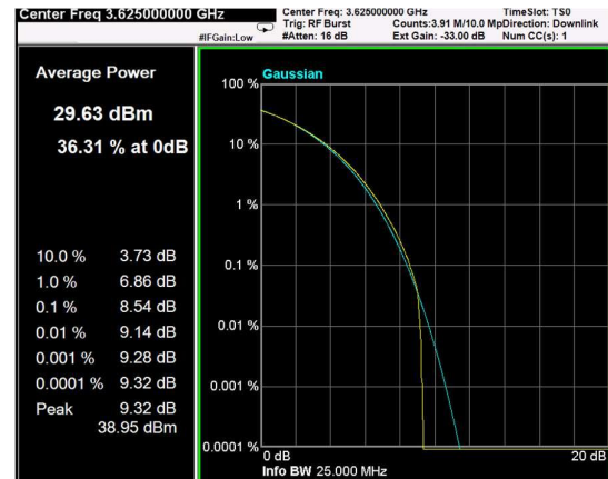
Channel: MIDDLE, Modulation: 256QAM, BW=10MHz, CCDF
