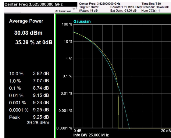
Channel: MIDDLE, Modulation: 16QAM, BW=10MHz, CCDF
