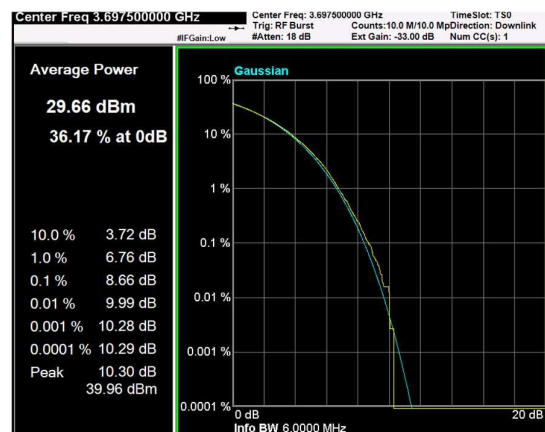
Channel: TOP, Modulation: 16QAM, BW=5MHz, CCDF
