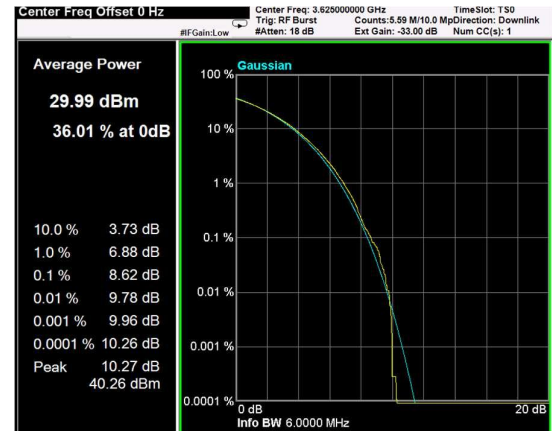
Channel: MIDDLE, Modulation: 256QAM, BW=5MHz, CCDF
