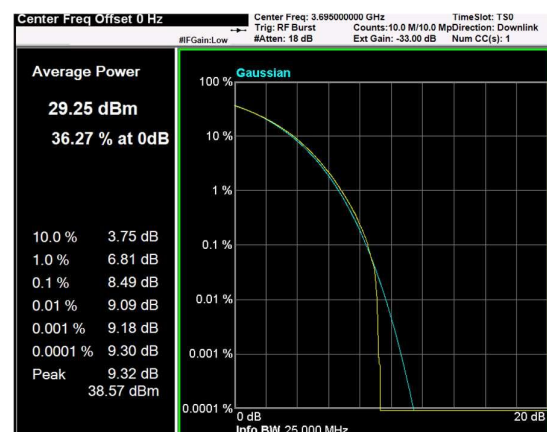
Channel: TOP, Modulation: 16QAM, BW=10MHz, CCDF
