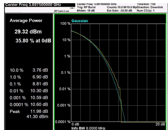
Channel: TOP, Modulation: 256QAM, BW=5MHz, CCDF
