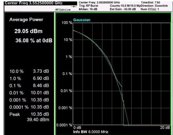
Channel: BOTTOM, Modulation: QPSK, BW=5MHz, CCDF
