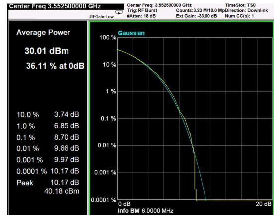
Channel: BOTTOM, Modulation: 256QAM, BW=5MHz, CCDF
