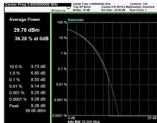
Channel: TOP, Modulation: 256QAM, BW=10MHz, CCDF
