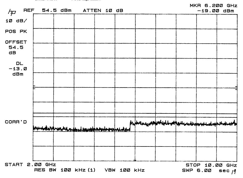
TEST: Conducted Spurious NOTE: Low Channel
