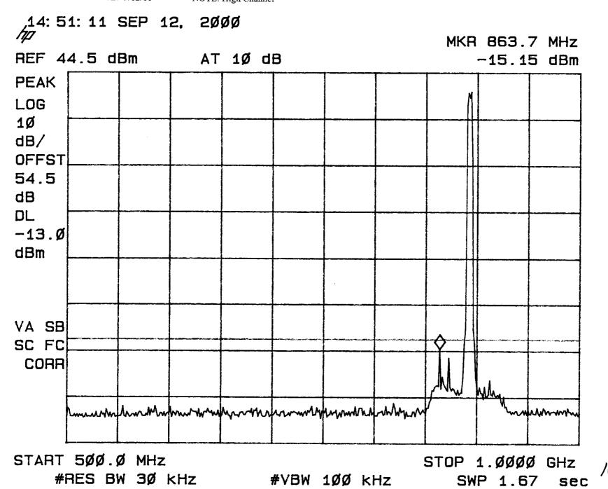
TEST: Conducted Spurious NOTE: High Channel
