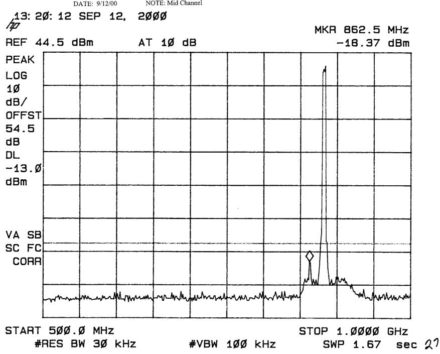
TEST: Conducted Spurious NOTE: Mid Channel
