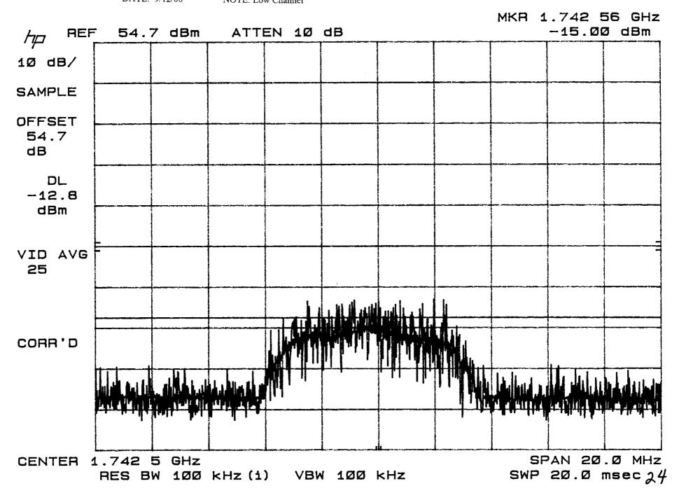
TEST: Conducted Spurious NOTE: Low Channel
