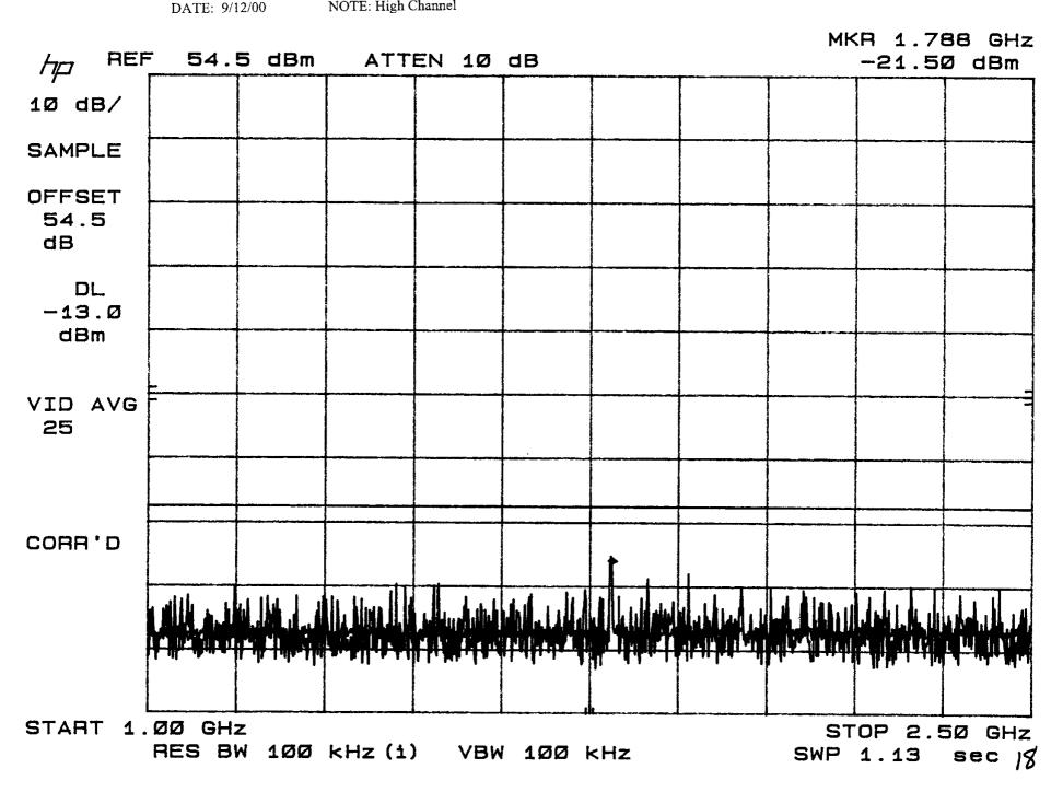
TEST: Conducted Spurious NOTE: High Channel
