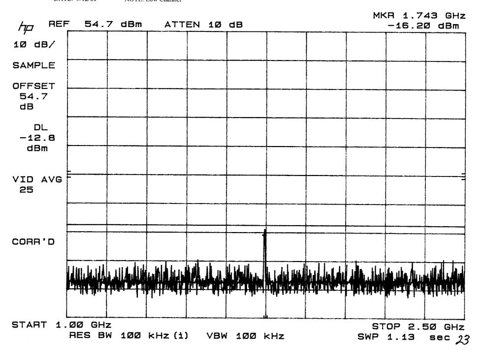
TEST: Conducted Spurious NOTE: Low Channel
