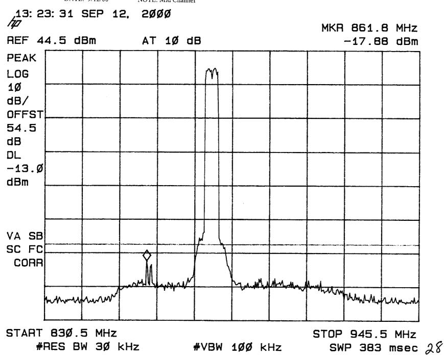
TEST: Conducted Spurious NOTE: Mid Channel
