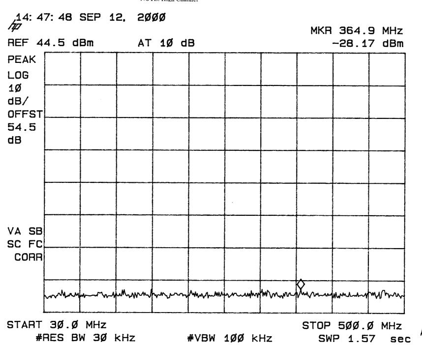
TEST: Conducted Spurious NOTE: High Channel
