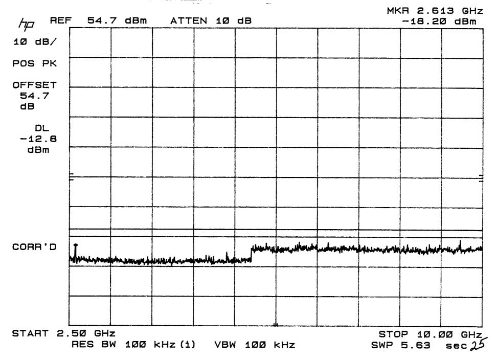
TEST: Conducted Spurious NOTE: Mid Channel
