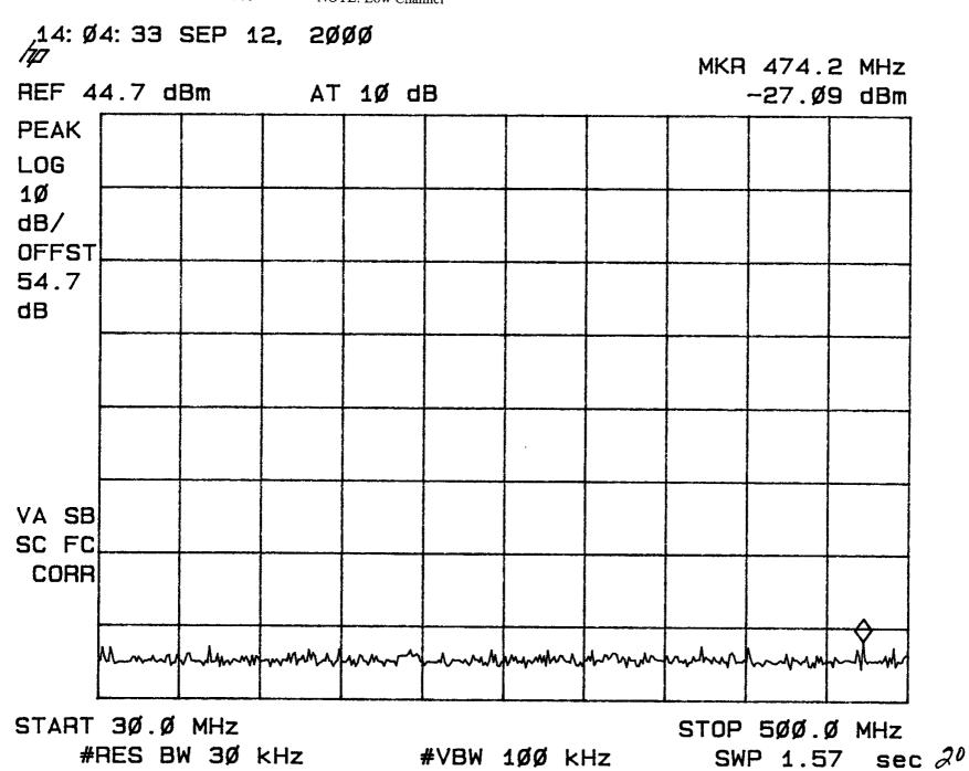
TEST: Conducted Spurious NOTE: Low Channel
