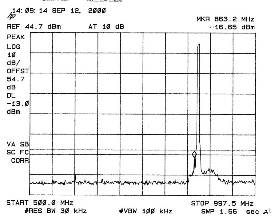
TEST: Conducted Spurious NOTE: Low Channel
