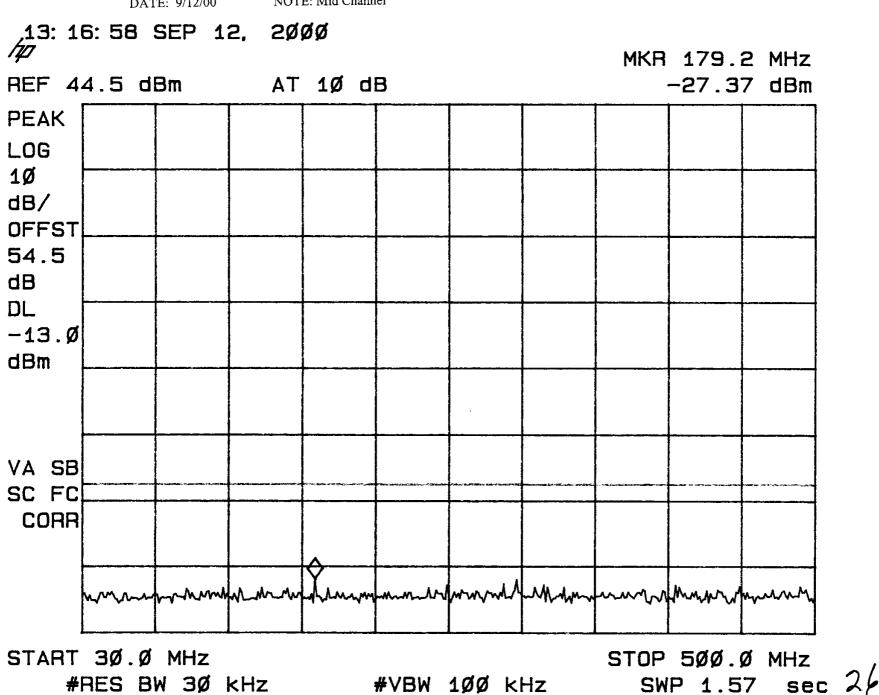
TEST: Conducted Spurious NOTE: Mid Channel
