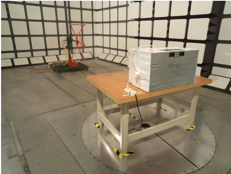
Radiated Emissions - Rear View (30 MHz – 1 GHz)
