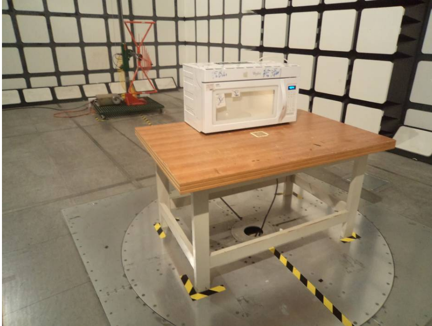
Radiated Emissions - Front View (30 MHz – 1 GHz)
