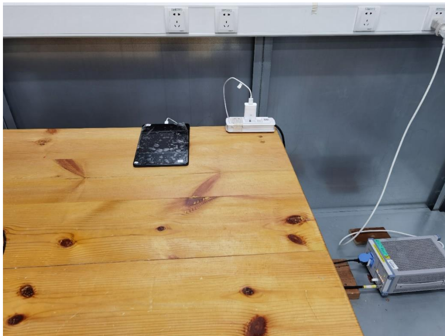
22. Conducted Emission (Part 15C, Bluetooth/Wi-Fi)
