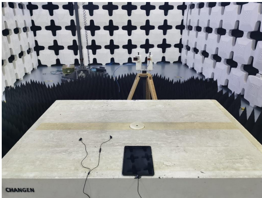
12. Radiated Emissions (Part 15B, FM receiver 26.5GHz-30GHz)
