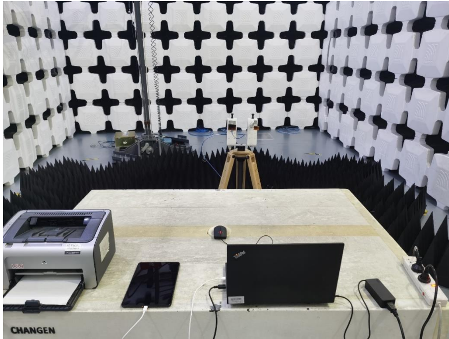
3. Radiated Emissions (Part 15B Data Transfer ,18GHz-26.5GHz)
