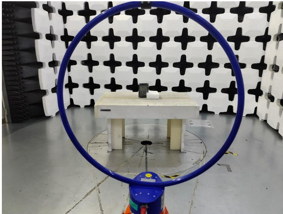
13. Radiated Emissions (Part 15C, 9kHz-30MHz)
