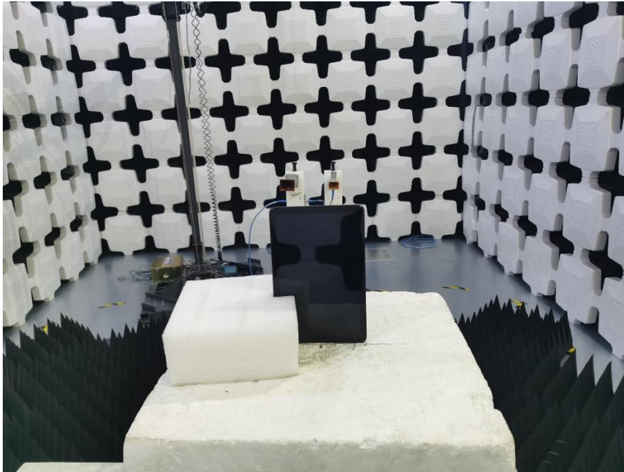
17. Radiated Emissions (Part 15C, 26.5GHz -40GHz)
