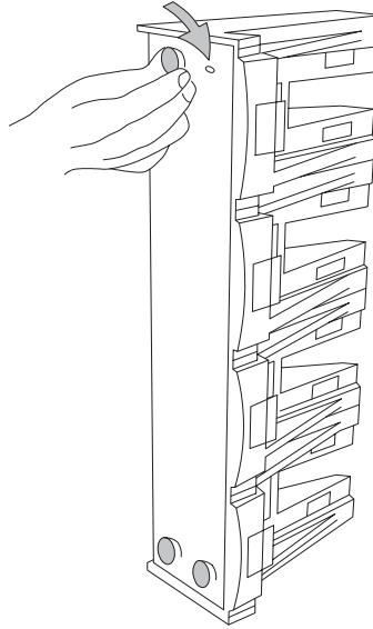
Figure 2-6. Installing Suction Cups on the CRD 38/6866
