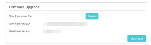
5. Wait a few minutes for the firmware upgrade to complete and the extender to reboot.
