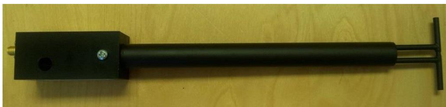
Figure 1 – MVG COMOSAR Validation Dipole
