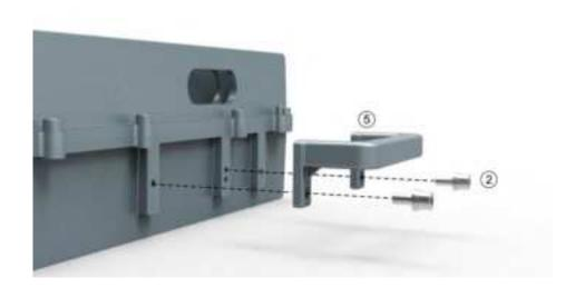
2. Attach and fasten the Bracket I to the back of HPRU with screws M6×14 using T5 Wrench.
