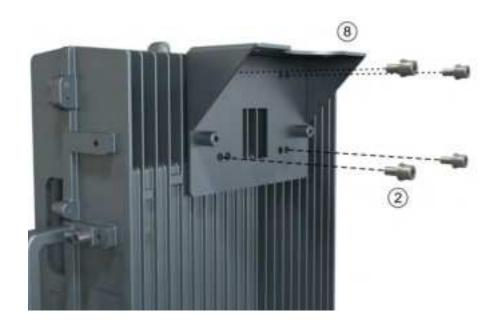
3. Mark the position of the drilling holes in the mounting Bracket II. Note: R = 13 mm.
