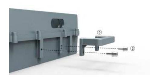
2. Attach and fasten the Bracket I to the left side of HPRU with screws M6×14 using T5 Wrench.
