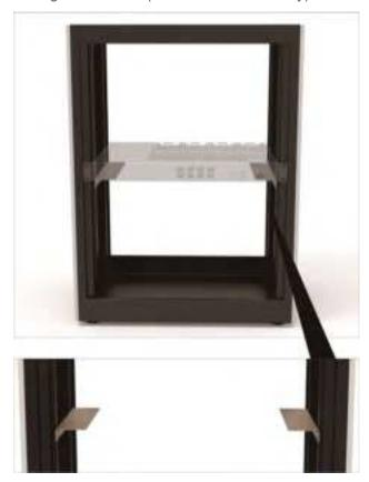
3. Place the AU in the rack and secure the AU using 2 screws M6×16 on both side and the Phillips screwdriver.
