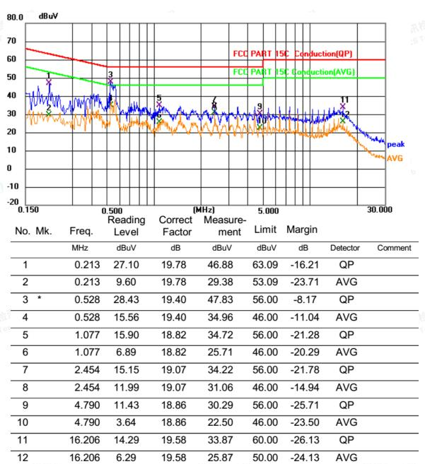
\*\*\*Note: Pre-scan all modes and recorded the worst case results in this report. Measurement= Reading + Correct Factor, Margin = Measurement - Limit. Correct Factor=Lisn Factor+Cable Factor+Insertion loss of Pulse Limiter
