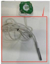
built-in temperature and humidity sensor
