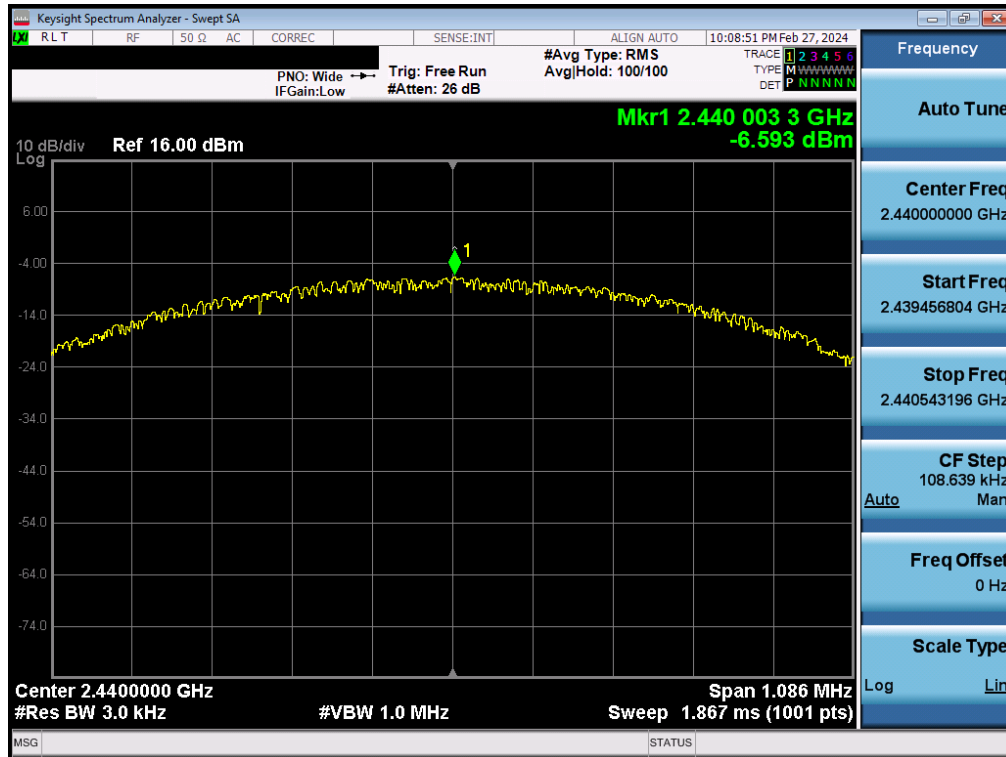
Plot 7-45. Power Spectral Density Plot Antenna 4a (Bluetooth (LE), 1Mbps, iPA – Ch. 19)
