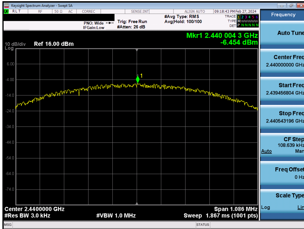
Plot 7-17. Power Spectral Density Plot Antenna 4a (Bluetooth (LE), 1Mbps, iPA – Ch. 19)
