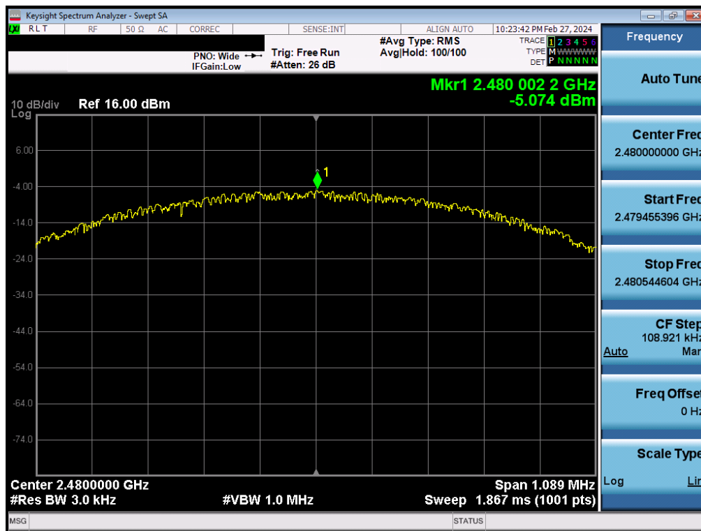
Plot 7-27. Power Spectral Density Plot Antenna 2a (Bluetooth (LE), 1Mbps, ePA – Ch. 39)
