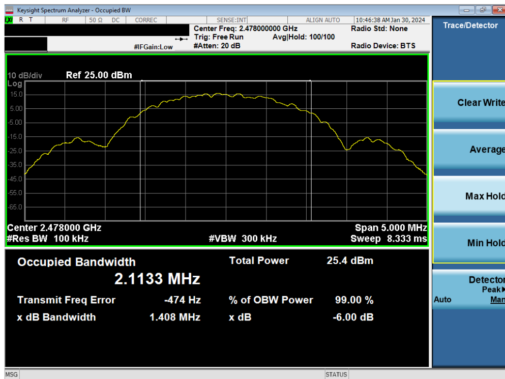
Plot 7-12. 6dB BW & 99% OBW Plot Antenna 2a (Bluetooth (LE), 2Mbps, ePA – Ch. 38)
