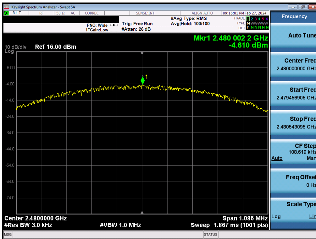
Plot 7-15. Power Spectral Density Plot Antenna 4a (Bluetooth (LE), 1Mbps, ePA – Ch. 39)
