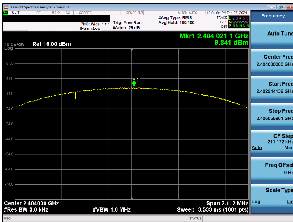
Plot 7-50. Power Spectral Density Plot Antenna 2a (Bluetooth (LE), 2Mbps, ePA – Ch. 1)
