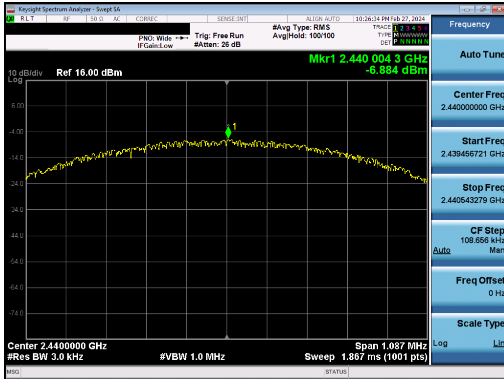
Plot 7-29. Power Spectral Density Plot Antenna 2a (Bluetooth (LE), 1Mbps, iPA – Ch. 19)
