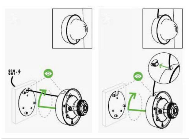
6. Place the camera over the top of the mount plate and match to plate hooks/mounts. Secure with Phillips or Torx head safety screw.
