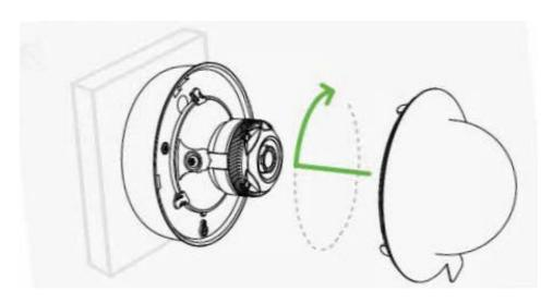
9. Remove the protective cover. The MV12 is equipped with a LED light on front of the unit to convey information about system functionality and performance.
