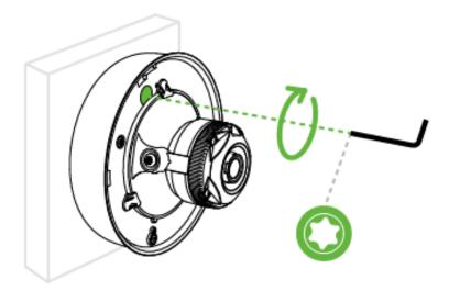
7. Aim the lens. Look through the camera on the Meraki Dashboard to fine tune the picture. The camera sensor and lens unit can be physically tilted through a range of 65 degrees, rotated through a range of 350 degrees, and panned through a range of 350 degrees. The image can only be rotated by 180 degrees in software and no other adjustments can be made. Zoom and focus can be adjusted remotely and cannot be adjusted physically on the camera.
