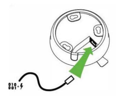
4. Remove the lens cover with protective shell still intact to connect the PoE RJ45 cable in two possible methods (1) through wall plate or (2) through the cable opening after removing the cable guard.
