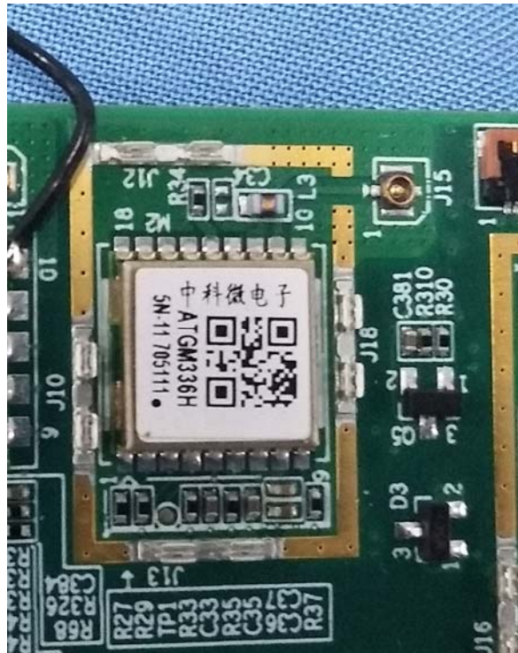
EUT – GPS Module View
