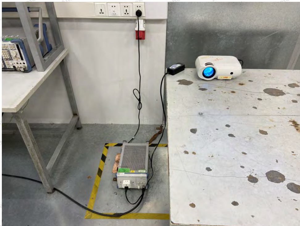
Photo of Power Line Conducted Emission Test
