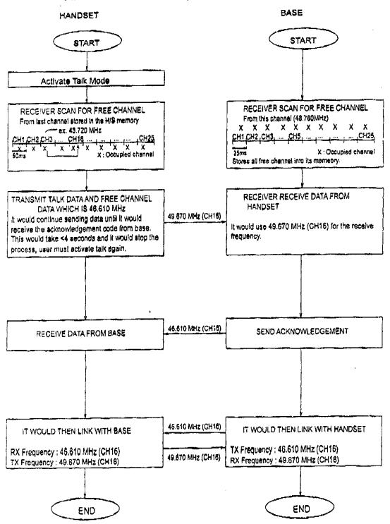
5. The test results demonstrating that this algorithm or program that is used to ensure that a link is not established on an occupied cordless telephone channel 1 through 15 are required by Section 15.333(b)(2)(i)
