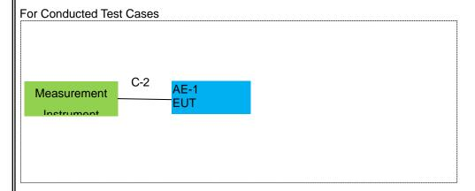
Note:1. The temporary antenna connector is soldered on the PCB board in order to perform conducted tests and this temporary antenna connector is listed in the equipment list. 2.EUT built-in battery-powered, the battery is fully-charged.
