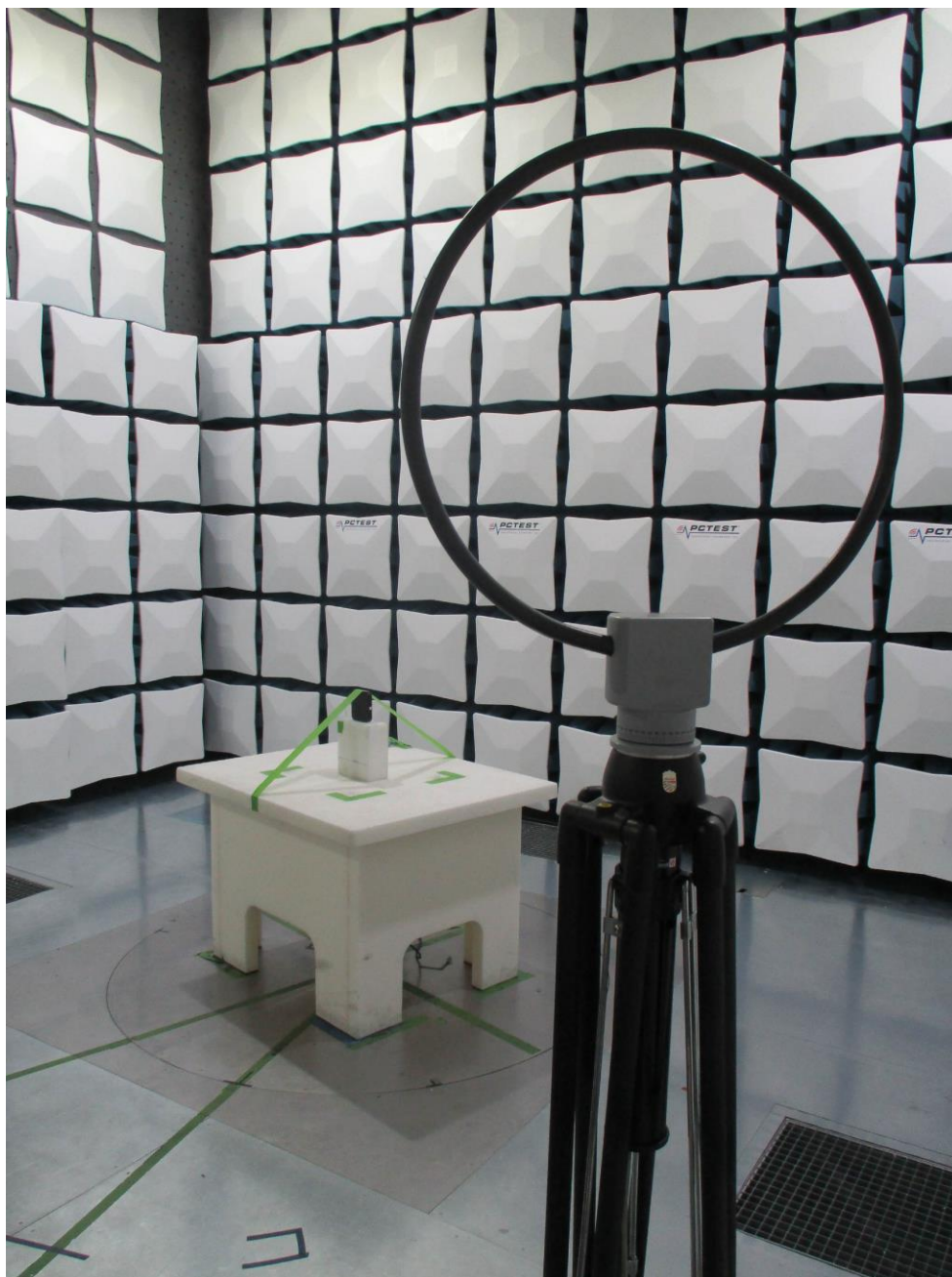
Figure7: 9kHz-30MHz Test Setup (Front View)
