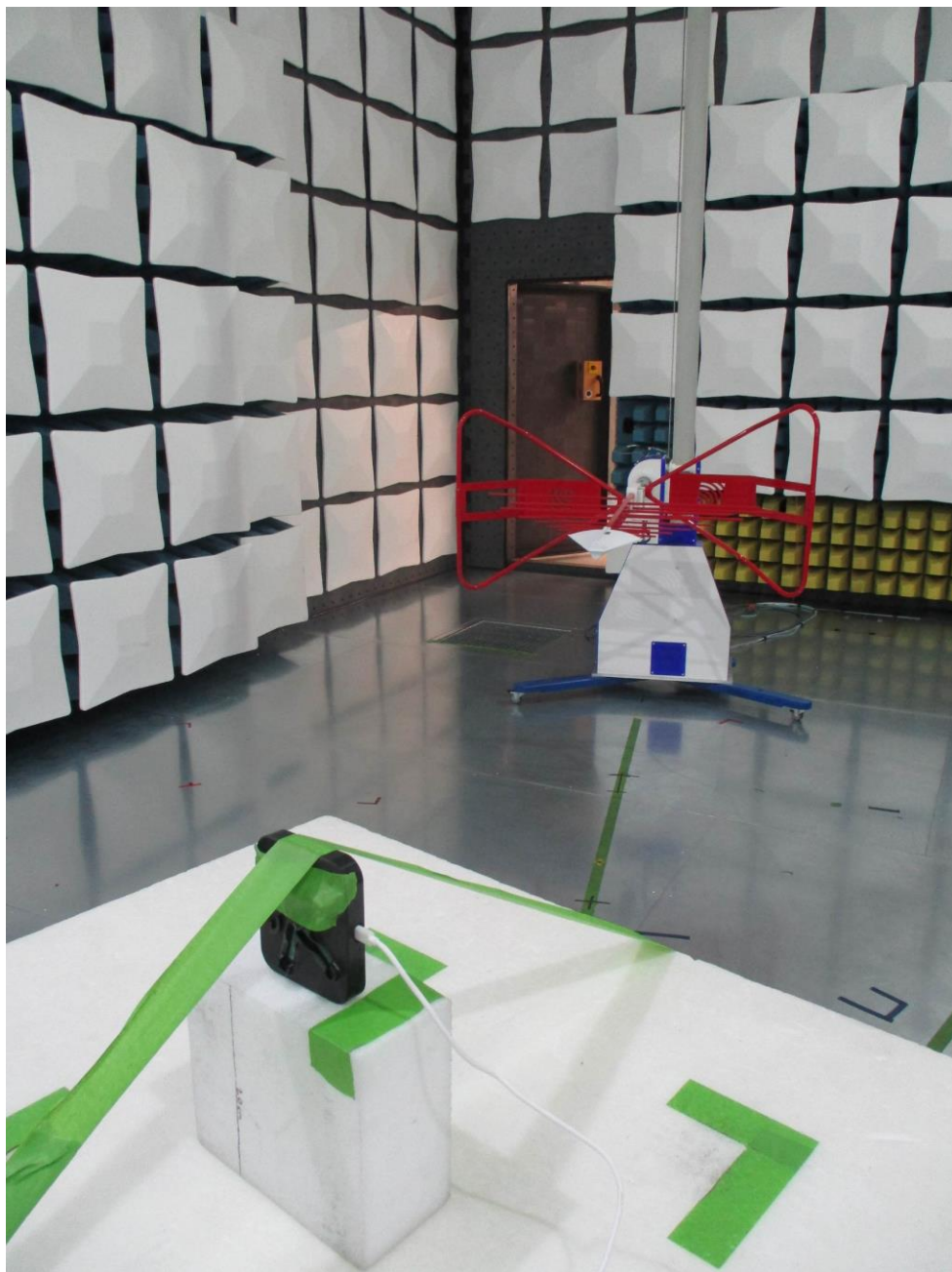
Figure 6: 30MHz-1GHz Test Setup (Rear View)
