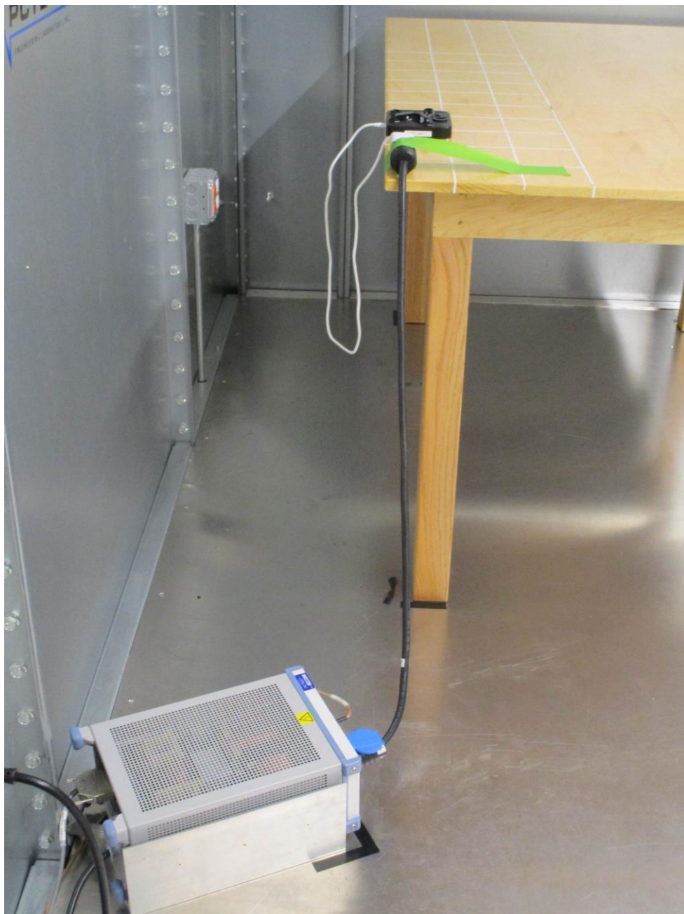
Figure 2: AC Line Conducted Emissions (Side View)
