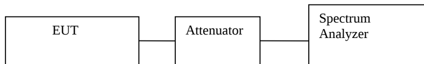
Figure 5. Block Diagram, Conducted Spurious Emissions Test Setup
