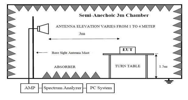
In Semi Anechoic Chamber (3m) Test Setup Diagram for Above 1GHz
