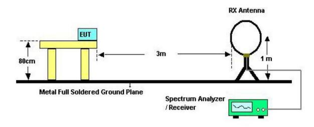
In Semi Anechoic Chamber (3m) Test Setup Diagram for 30MHz~1000MHz
